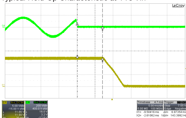
Typical Hold-Up Characteristic at 115 Vin
